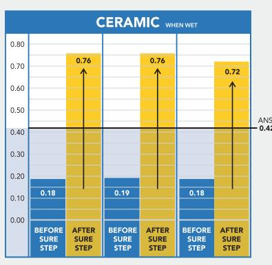
SSI, NY conducted testing at the RSI Tribological Lab, TX, according to The American National Standard Institute (ANSI) A326.3, "Test Method for Measuring Dynamic Coefficient Of Friction (DCOF) of Hard Surface Floor Materials." The above charts represent the average result of thirty-six (36) dynamic measurements that were taken on each of the porcelain and ceramic tiles. All data was recorded.
